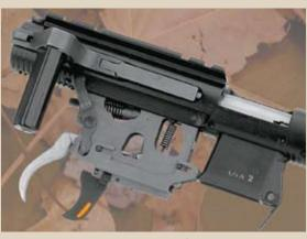
The sample rifle's trigger broke at 2½ lbs., which contributed to the rifle's accuracy. The safety is actually in the front of the trigger guard, much like an M1 Garand.
