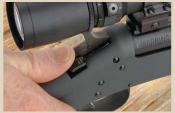
Functionally and cosmetically there are no surprises with the .17 HMR Sportster. Its matte-blue break-open action retains the familiar side-lever barrel release and exposed hammer.
