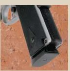
Smith & Wesson uses several recognizable aftermarket parts in its 1911 pistol. An example of that is the machined aluminum mainspring housing (r.), which is used instead of an equivalent plastic part seen on many other pistols. The stainless steel barrel has a slightly oversize area near the muzzle to promote a better barrel to bushing fit (l.). The fit of the bushing to the slide does not necessitate a wrench for turning, but is not overly loose, either.
