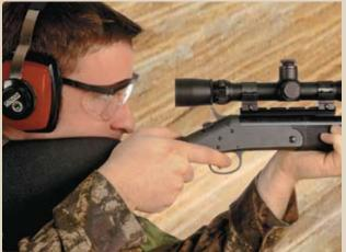
Aiding accurate shooting is a Monte Carlo comb on the black, high-density polymer stock that helps position the shooter's eye directly in line with the scope.
