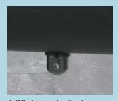
A QD stud under the freefloating fore-arm allows for instant attachment/detachment of a bipod.
